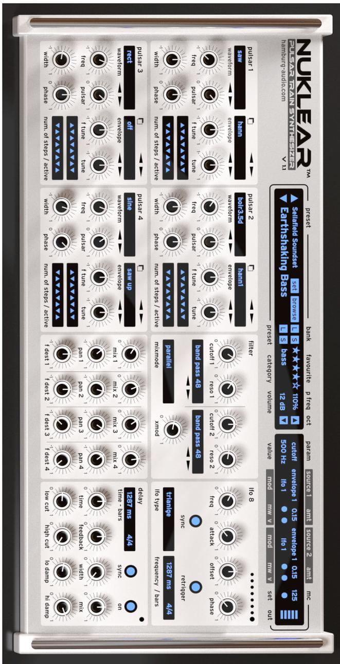
Fig. 4. Graphical user interface of *Nuklear*, a plug-in synthesiser based on Pulsar Synthesis
